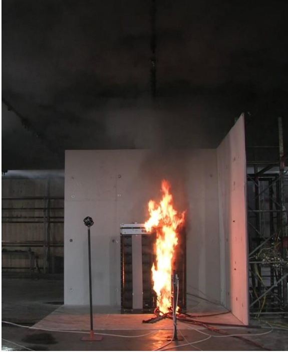
Figure 6-20: Photos of LFP sprinklered test during fire development: first sprinkler operation (left) and peak heat release rate (right).
