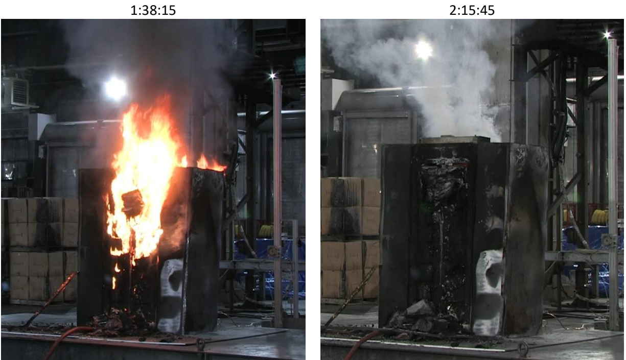
Figure 6-4: Photos of LFP fire during decay phase (left) and at self-extinguishment (right).
