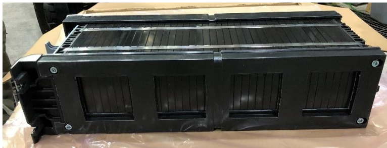
Figure 3-2: Photos of LFP module with front face of module shown on left side of picture.
