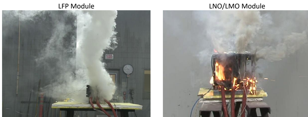
Figure 4-6: Example of LFP (left) and LNO/LMO (right) battery response to abuse conditions. LFP batteries vented a thick white smoke and sometime required an external pilot flame to ignite, whereas LNO/LMO batteries generate sparks that consistently ignited vent gases.
