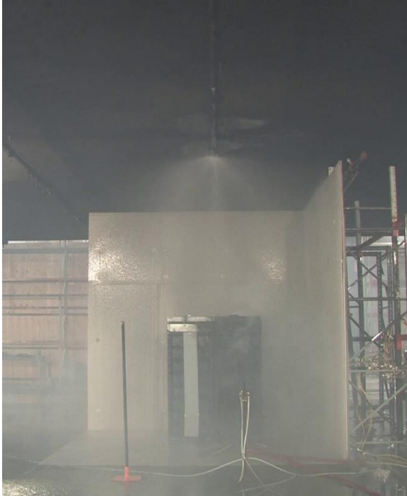
Figure 6-21: Photos of LFP sprinklered test during fire decay phase (left) and at burnout (right).
