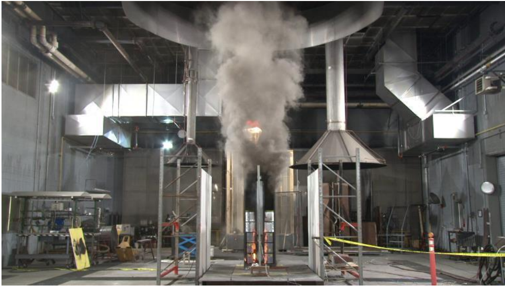
Figure 5-1: Image of six-module fire test with LNO/LMO module
