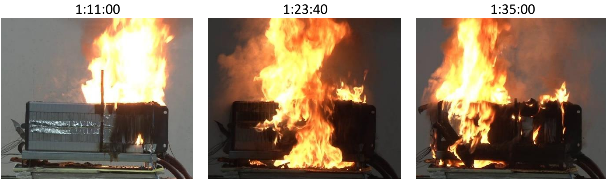
Figure 4-7: Side view of lateral fire propagation for LNO/LMO module; in this view the ignition heaters are located on the right half (front) of the module and the fire progress from the right to left.
