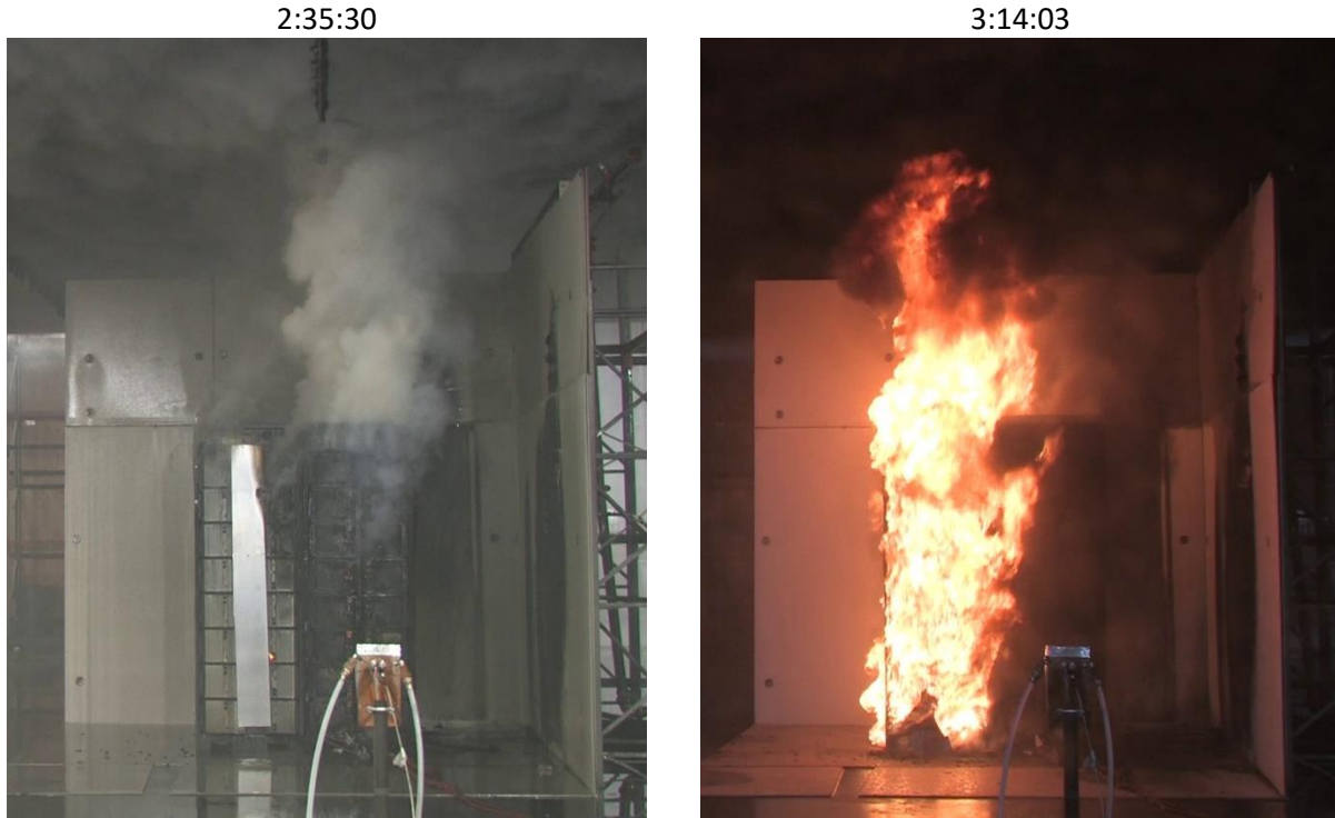
Figure 6-23: Photos of LNO/LMO sprinklered test during fire development on target rack: view of rack once sprinklers were shut off (left) and fire size when sprinklers were turned back on (right).
