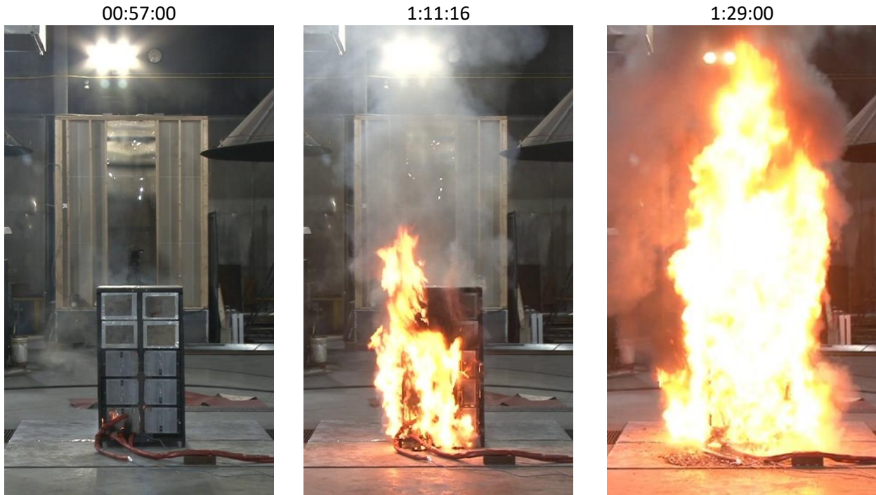
Figure 5-5: Photos of LNO/LMO fire development during intermediate-scale free burn test: near time of ignition (left), near time of predicted sprinkler operation (middle), peak heat release rate (right).
