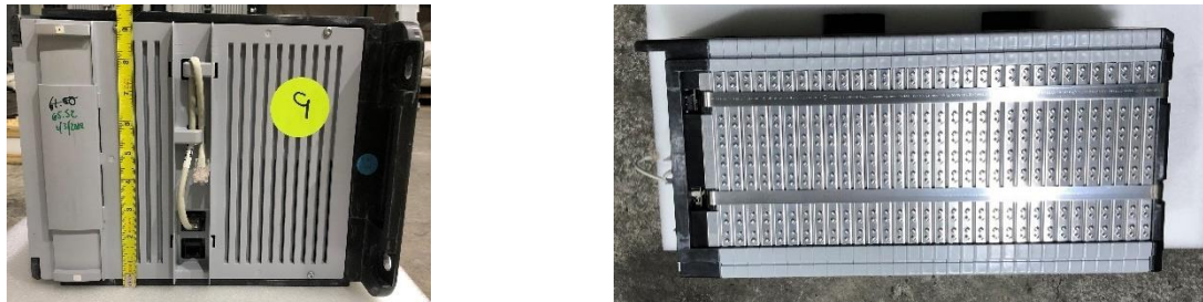
Figure 3-4: Photos of LNO/LMO module; front face (left) and top with front face of module shown on left side of picture (right)
