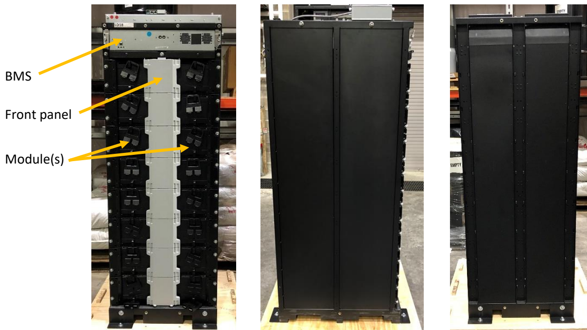
Figure 3-1: Photos of LFP rack; front (right), side (middle), and back (left).
