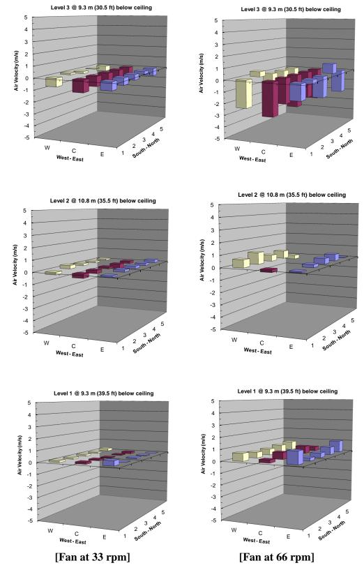
Figure 5-11: Air velocity through array with the fan at 33 and 66 rpm for Test 4 [no fire]
