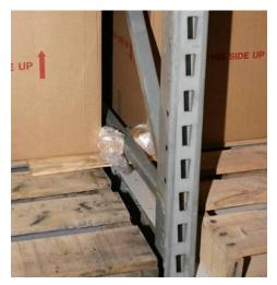
Figure 4-6: Igniters within the rack, located at the rack uprights
