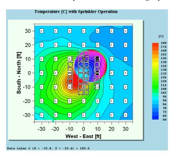
Figure B-7: Ceiling TC contours at first sprinkler operation (1 min 28 s) – Test 1
