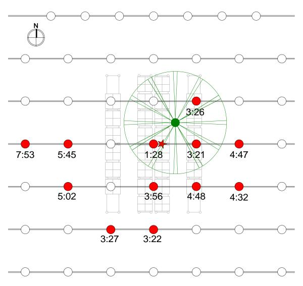
Figure B-1: Plan view of sprinkler operation pattern - Test 1
