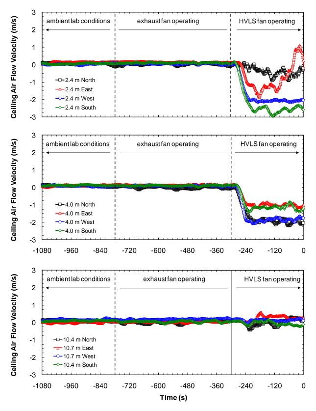
Figure 5-4: Ceiling level air flow resulting from building exhaust only for Test 1
