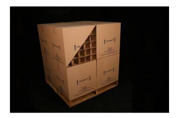
Figure 4-2: Photo of cartoned unexpanded plastic (CUP) commodity
