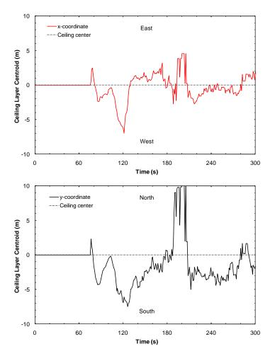
Figure E-6: Time evolution of x- and y-coordinate of ceiling layer centroid – Test 4
