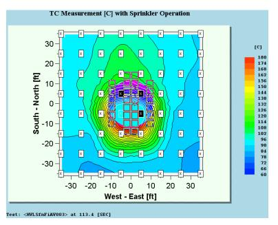
Figure D-7: Ceiling TC contours at first sprinkler operation (1 min 54 s) – Test 3
