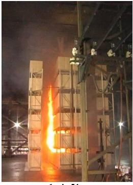
1 min 42 s1 min 54 s[1<sup>st</sup> sprinkler activation in Test 2][1<sup>st</sup> sprinkler operation in Test 3]Figure 6-1: Photos of Test 2
