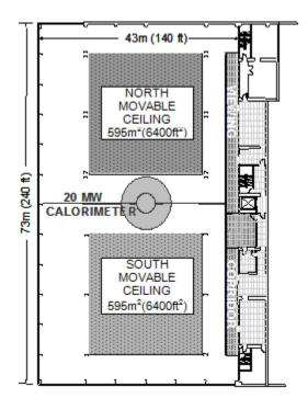
Figure 4-1: Illustration of FM Global Large Burn Laboratory test locations
