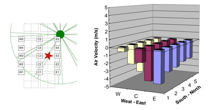
Figure 5-5: Air-flow at top of array [3.2 m (10.5 ft) below ceiling] with fan operating at 66 rpm for Test 1
