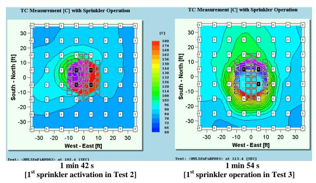
Figure 6-4: Ceiling TC measurement contour plot for Test 3
