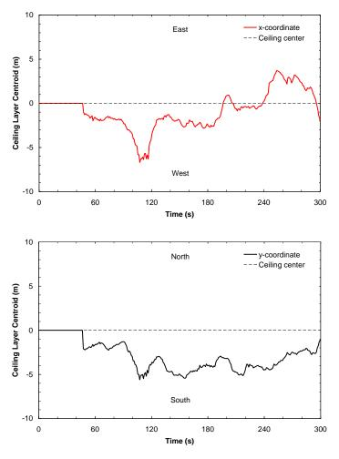
Figure B-6: Time evolution of x- and y-coordinate of ceiling layer centroid – Test 1
