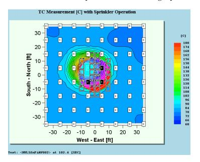
Figure C-7: Ceiling TC contours at first sprinkler operation (1 min 42 s) – Test 2
