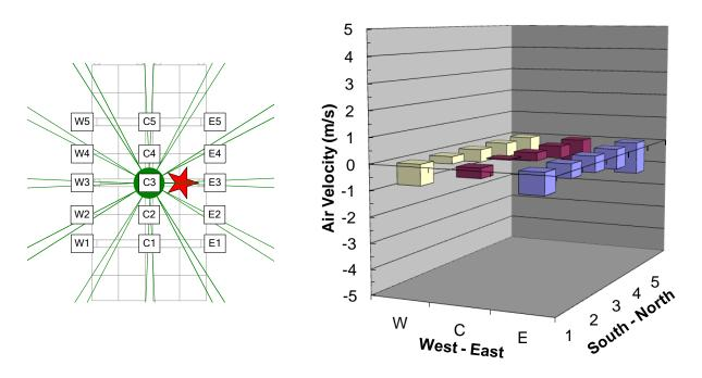
Figure 5-8: Air-flow at top of array [7.8 m (25.5 ft) below ceiling] with fan operating at <u>33 rpm</u> for Test 4
