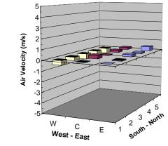
Figure 5-9: Air velocity through array with the fan at 66 rpm for Test 1 [no fire]
