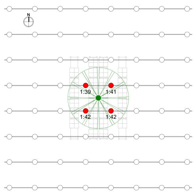
Figure E-1: Plan view of sprinkler operation pattern - Test 4
