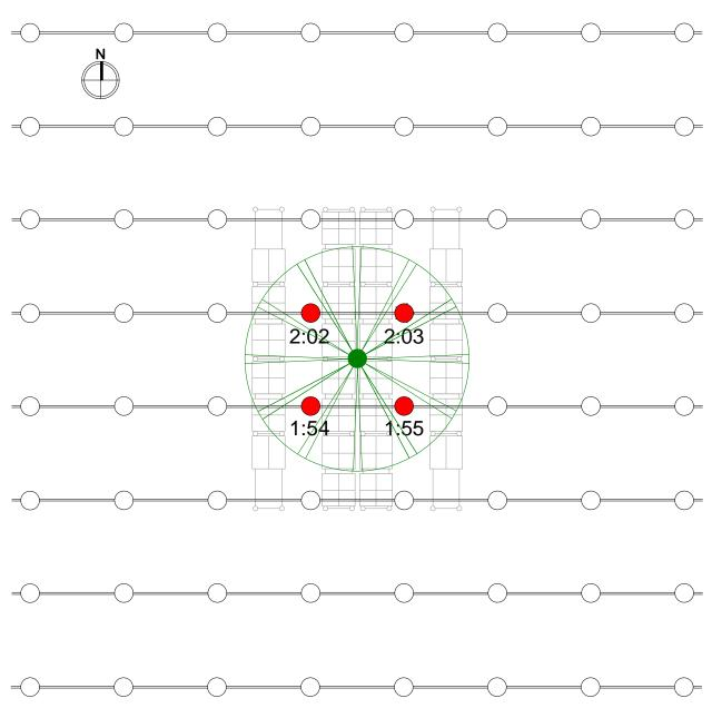
Figure D-1: Plan view of sprinkler operation pattern - Test 3
