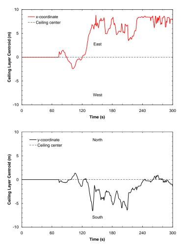
Figure D-6: Time evolution of x- and y-coordinate of ceiling layer centroid – Test 3
