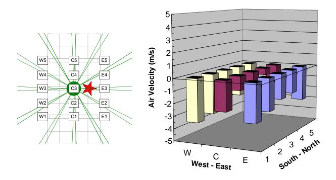
Figure 5-6: Air-flow at top of array [3.2 m (10.5 ft) below ceiling] with fan operating at 66 rpm for Tests 2 and 3
