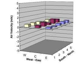
Figure 5-10: Air velocity through array with the fan at 66 rpm for Tests 2 and 3 [no fire]
