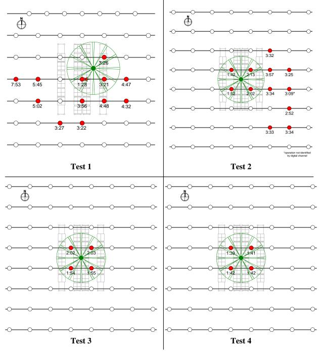
Figure 5-1: Sprinkler operation pattern for Tests 1 - 4
