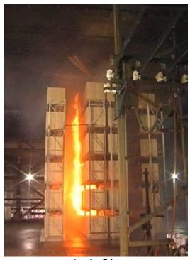
1 min 42 s1 min 54 s[1<sup>st</sup> sprinkler activation in Test 2][1<sup>st</sup> sprinkler operation in Test 3]Figure 6-2: Photos of Test 3
