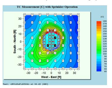
Figure E-7: Ceiling TC contours at first sprinkler operation (1 min 39 s) – Test 4
