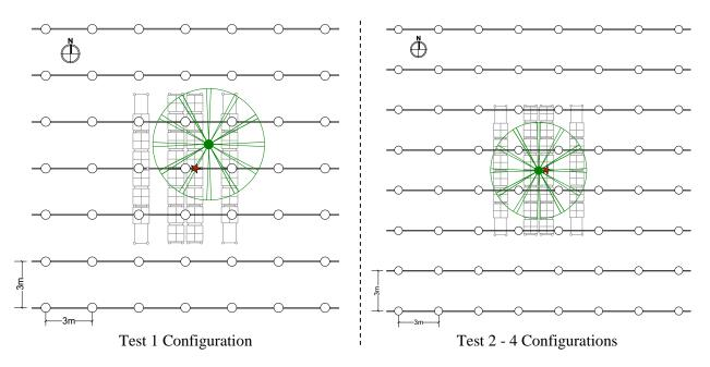
Figure 4-7: Sprinkler layout for Tests 1 – 4
