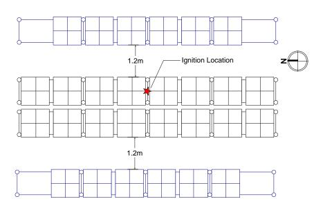
Figure 4-4: Plan view of main and target arrays
