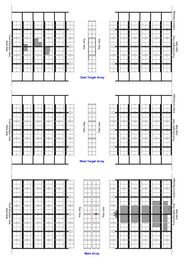
Figure D-2: Damage assessment - Test 3
