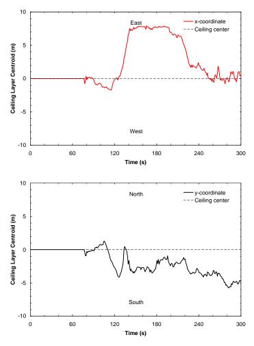
Figure C-6: Time evolution of x- and y-coordinate of ceiling layer centroid – Test 2
