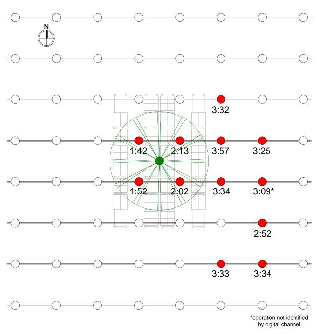
Figure C-1: Plan view of sprinkler operation pattern - Test 2
