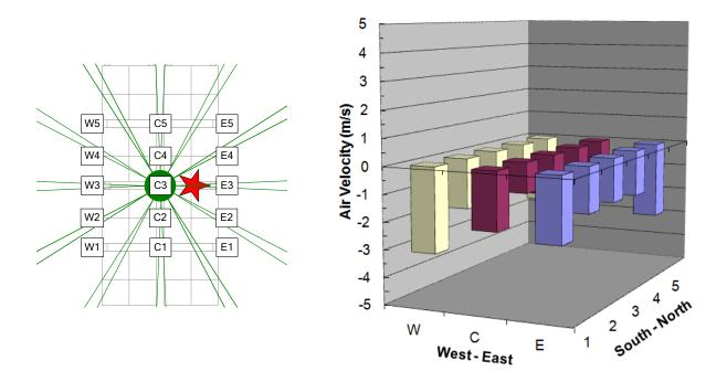
Figure 5-7: Air-flow at top of array [7.8 m (25.5 ft) below ceiling] with fan operating at <u>66 rpm</u> for Test 4
