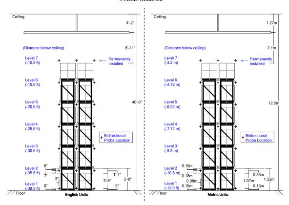
Figure 4-10: Supplementary air-flow measurements within main array for Tests 2 and 3 configuration (English and metric units)
