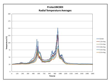
Figure A-5: Test 3 - Ceiling Gas Temperatures
