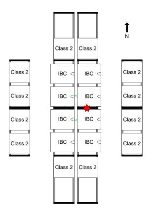
Figure 2-8: Schematic Plan View of Rack Storage Empty IBC Array
