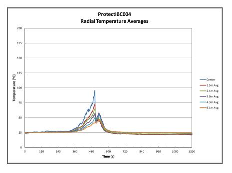
Figure A-7: Test 4 - Ceiling Gas Temperatures
