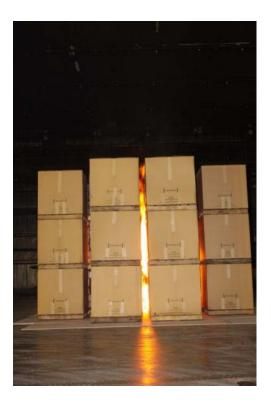
Figure 3-21: Photo of Test Array just Prior to 1<sup>st</sup> Sprinkler Operation (Test 4)
