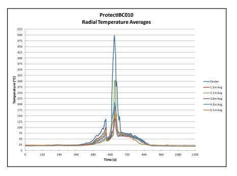
Figure A-9: Test 10 - Ceiling Gas Temperatures
