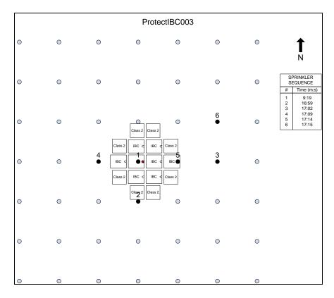
Figure 3-13: Test 3 - Sprinkler Operation Pattern
