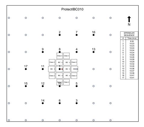
Figure 3-26: Test 10 - Sprinkler Operation Pattern
