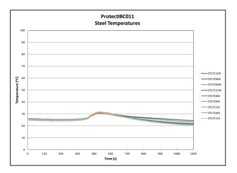
Figure A-12: Test 11 - Ceiling Steel Temperatures
