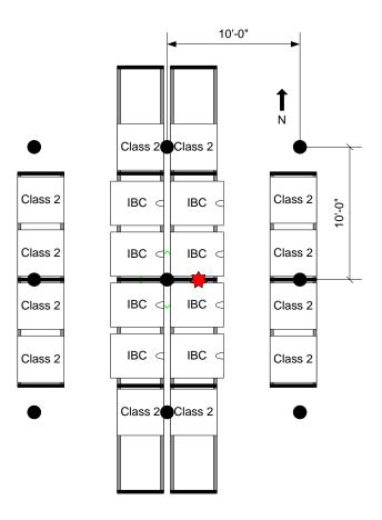
Figure 2-13: Igniter/Sprinkler Location for Rack Storage Empty IBC Test Array
