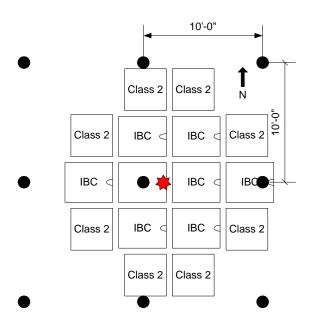
Figure 2-12: Igniter/Sprinkler Location for Stacked Empty IBC Test Array
