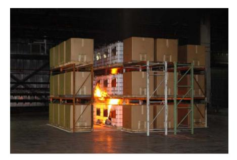
Figure 3-33: Photo of Array Prior at 1<sup>st</sup> Sprinkler Operation ~7 min 28 s (Test 11)
