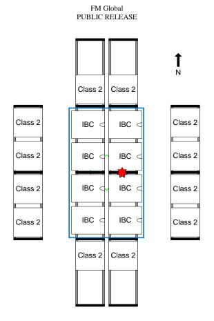
Figure 2-17: Acceptable Damage Area for Rack Storage Array
