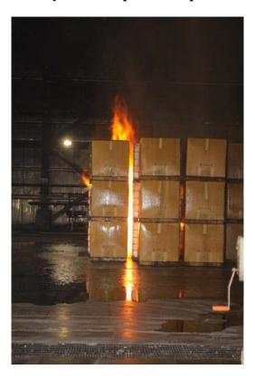
Figure 3-15: Photo of Array at ~16 min 38 s (Test 3)
