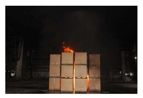
Figure 3-8: Photo of Array at 1<sup>st</sup> Sprinkler Operation (Test 2)
