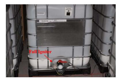
Figure 2-14: Photo of Igniter Placement for Stacked IBC Tests
