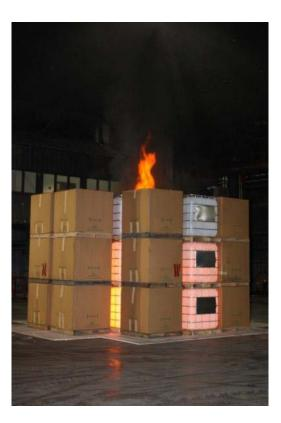
Figure 3-27: Photo of Array Prior at 1<sup>st</sup> Sprinkler Operation ~9 min 30 s (Test 10)
