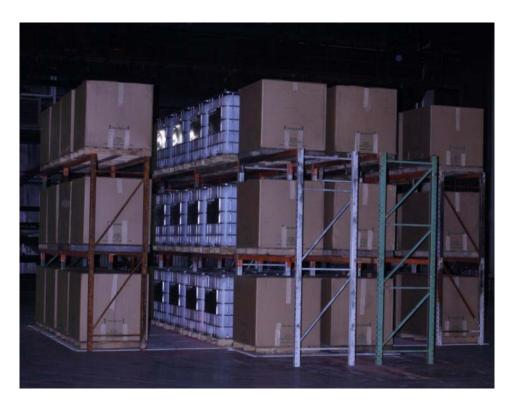
Figure 2-9: Photo of Rack Storage IBC Array
