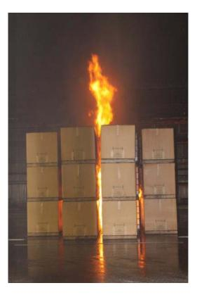
Figure 3-14: Photo of Array after 1<sup>st</sup> Sprinkler Operation ~9 min 40 s (Test 3)
