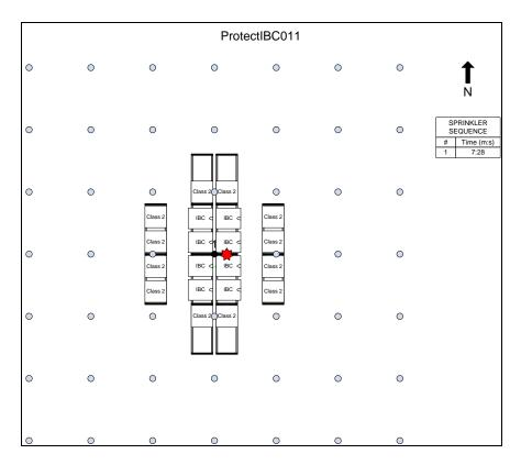
Figure 3-32: Test 11 - Sprinkler Operation Pattern
