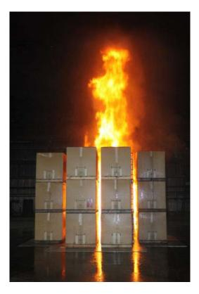
Figure 3-28: Photo of Array Prior to 2<sup>nd</sup> Sprinkler Operation ~10 min 12 s (Test 10)
