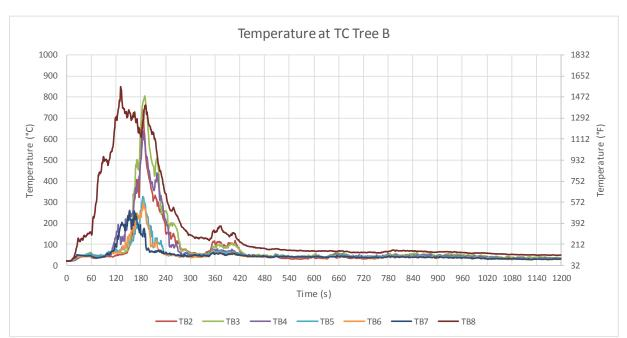
Figure B-29: Test 1 temperatures at TC Tree B. TC TB1 malfunctioned and the data is not presented. Increase in temperature at TB2-TB7 after 01:40 is likely due to the arrival of the flame front. Their magnitude prior to this time are an indication of vertical temperature profiles not directly exposed to the fire plume. In hindsight it would have been advantageous to install a TC tree in the aisle space between Sides B and D to provide gas temperature for regions not directly exposed to the fire.
