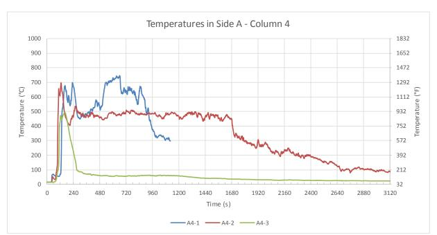
Figure B-39: Test 2 temperatures in Side A: Column 4. Note that TC A4 -1 malfunctioned during the test and suspect data have not been plotted. Its functionality was checked post-test and found to be inoperative.
