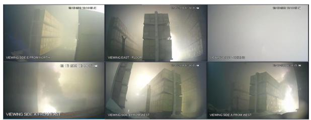
Figure A-12: Test 1 at 02:30: sprinklers continue to operate; the fire involves Side A and C.
