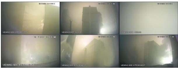
Figure A-13: Test 1 at 03:00: all 35 sprinklers have operated, sparks have been showering the lab since 00:33, visibility is decreasing.
