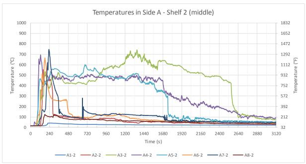
Figure B-34: Test 2 temperatures in Side A: Shelf 2 (middle).
