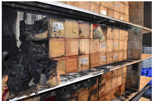
Figure C-12: Test 1, west side of Shelves 3, 4 and 5 in Side C showing examples of locations where flame spread ceased in the absence of a flame break. Shelf 3 provides an example of the flame spread that occurs when the flames are channeled along the underside of the shelves.
