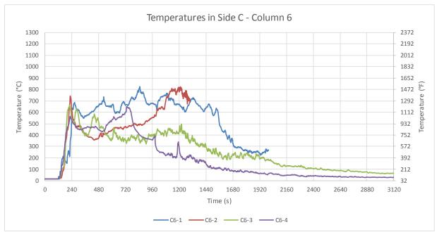
Figure B-54: Test 2 temperatures in Side C: Column 6. Note that TCs C6-1 and C6-2 malfunctioned during the test and suspect data have not been plotted. Their functionality was checked post-test and found to be inoperative.
