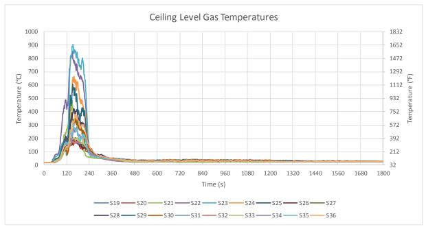
Figure B-31: Test 2 ceiling-level gas temperatures at TC locations 19-36.
