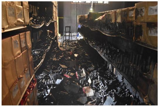
Figure C-4: Test 1 damage to Sides A (right) and C (left), looking toward west, with collapsed commodity in aisle which occurred during the test and not as a result of firefighting efforts.
