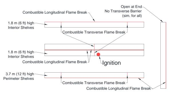
Figure 2-2: Plan view of shelving unit showing flame break locations.
