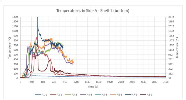
Figure B-33: Test 2 temperatures in Side A: Shelf 1 (bottom). Note that TCs A3-1, A4-1, A5-1, A6-1 and A7-1 malfunctioned during the test and suspect data have not been plotted. A7-1 exceed the maximum rating of a Type K TC at 06:10 after which time the temperature decreased. Their functionality was checked post-test and found to be inoperative. Note different temperature scale.
