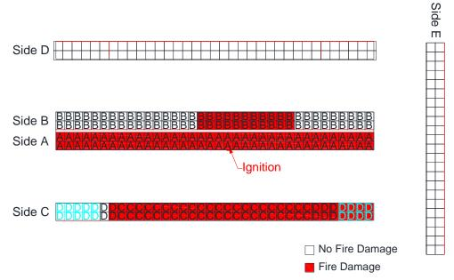
Figure 3-8: Test 2 plan view of maximum extent of fire damage.
