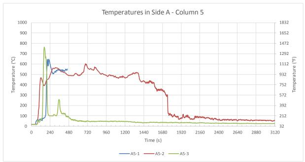
Figure B-40: Test 2 temperatures in Side A: Column 5. Note that TC A5-1 malfunctioned during the test and suspect data have not been plotted. Its functionality was checked post-test and found to be inoperative.
