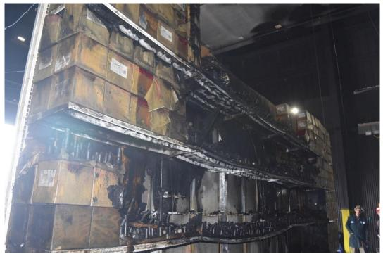
Figure C-23: Test 2 Side C looking toward west, shelves 3-5, transverse flame break on shelves 4 and 5 (top) intact.
