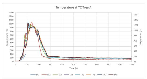
Figure B-57: Test 2 temperatures at TC Tree A. Note that TCs TA1 and TA4 malfunctioned during the test and suspect data have not been plotted. Their functionality was checked posttest and found to be inoperative. High temperatures are a result of the proximity of the fire to the TC tree and are not indicative of vertical temperature profiles in other regions of the test array. Note different temperature scale.
