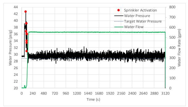
Figure 3-7: Test 2 water pressure and flow rate.
