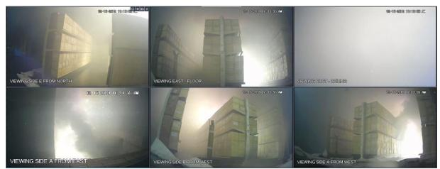
Figure A-11: Test 1 at 02:20: sprinklers continue to operate, ceiling-level gas temperatures (refer to Appendix B) are roughly steady state at maximum values.
