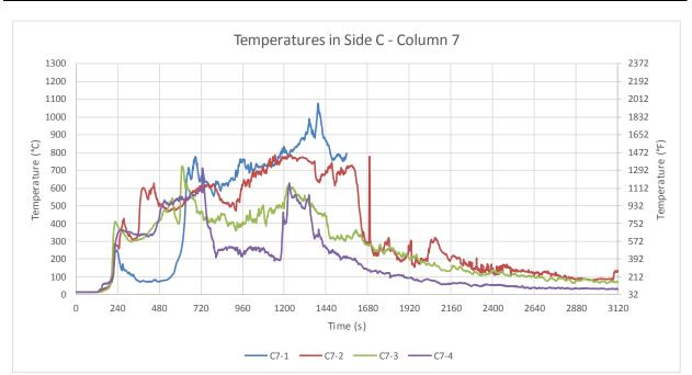
Figure B-55: Test 2 temperatures in Side C: Column 7. Note that TCs C7-1 and C7-2 malfunctioned during the test and suspect data have not been plotted. Their functionality was checked post-test and found to be inoperative.
