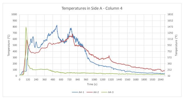
Figure B-10: Test 1 temperatures in Side A: Column 4.
