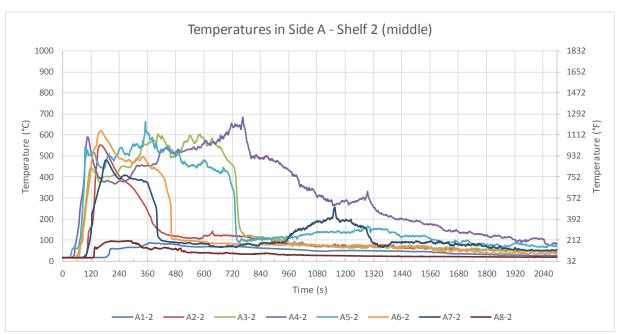
Figure B-5: Test 1 temperatures in Side A: Shelf 2 (middle).
