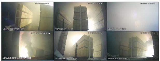
Figure A-9: Test 1 at 02:00: sprinklers continue to operate, fire and smoke production intensifying.
