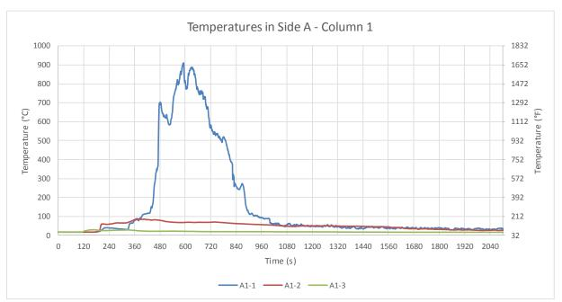
Figure B-7: Test 1 temperatures in Side A: Column 1.
