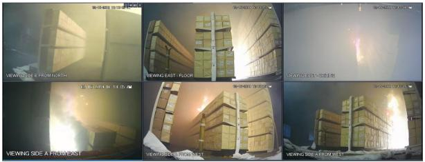
Figure A-6: Test 1 at 01:30: four sprinklers operating, fire and smoke production intensifying in Side A.
