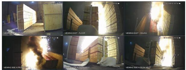
Figure A-24: Test 2 at 01:30: 2 s after 1<sup>st</sup> sprinkler activation, fire and smoke production intensifying, fireworks on top shelf of Side B became active at 01:23.
