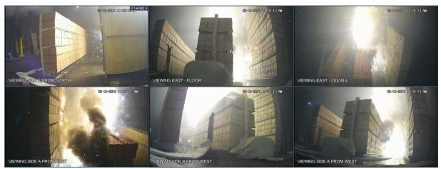
Figure A-26: Test 2 at 01:50: four sprinklers operating and fire and smoke production continue to intensify.
