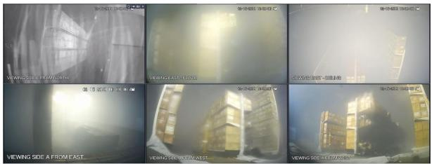
Figure A-18: Test 1 at 28:00: camera 1 in infrared shows water droplets, cameras 2, 5 and 6 show fire damage in bottom and middle shelf of Side A.
