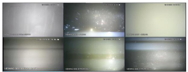
Figure A-16: Test 1 at 05:10: lab visibility completely obscured, camera 1 had transitioned to black and white colored infrared, cameras 2, 5 and 6 showing sparks visible in dark lab space.
