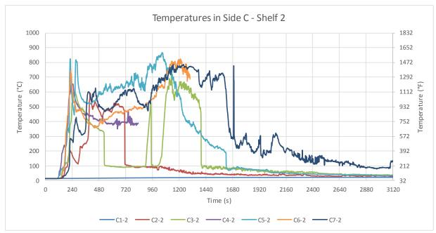
Figure B-46: Test 2 temperatures in Side C: Shelf 2. Note that TCs C4-2, C6-2 and C7-2 malfunctioned during the test and suspect data have not been plotted. Their functionality was checked post-test and found to be inoperative.
