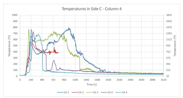
Figure B-52: Test 2 temperatures in Side C: Column 4. Note that TCs C4-1 and C4-2 malfunctioned during the test and suspect data have not been plotted. Their functionality was checked post-test and found to be inoperative.
