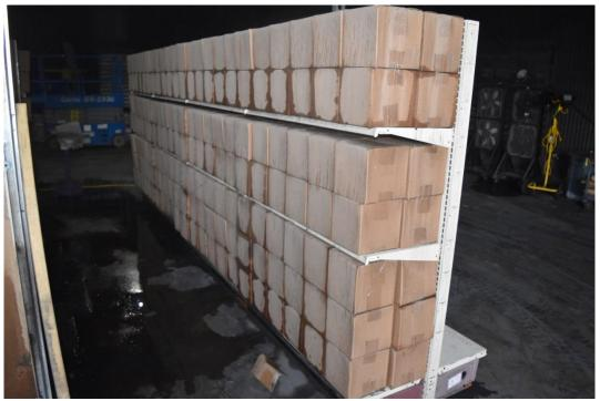
Figure C-31: Test 2 post-test image of Side E which sustained water damage only (no fire).
