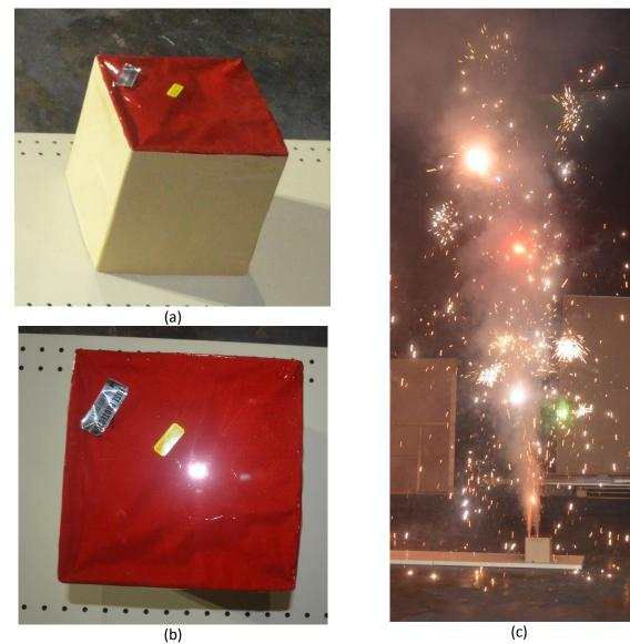
Figure 2-14: Single device (a) side and top, (b) cellophane top showing fuse, (c) example of one phase of discharge of device, display reaches approximately 4.9 m (16 ft) high.
