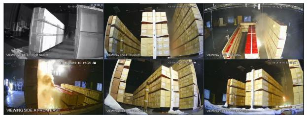
Figure A-2: Test 1 at 00:50: fire and smoke production intensifying in ignition region.
