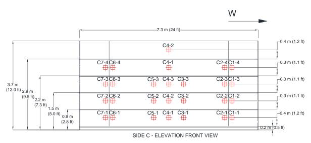
Figure 2-5: Front elevation view of Side C showing shelf height and thermocouple nomenclature and vertical dimensions of locations. Red crosses represent TCs.
