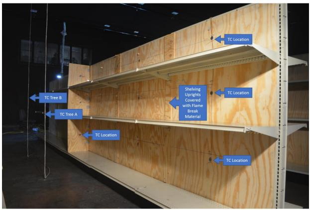
Figure 2-11: Shelving construction showing examples of TC locations, covering of penetrations in rack uprights with flame break material and TC Tree locations.
