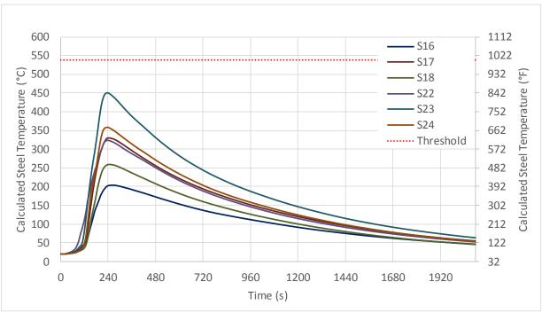
Figure 3-5: Test 1 calculated ceiling-level steel temperatures for locations where gas temperatures exceeded 538°C (1000°F).
