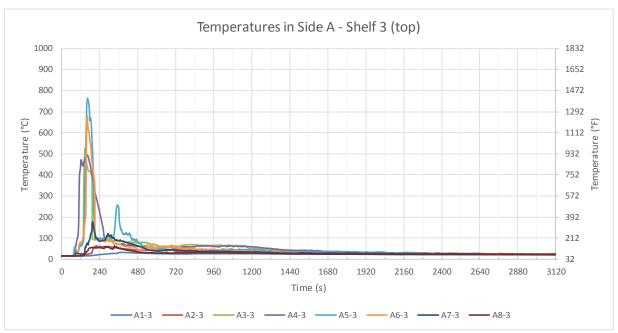
Figure B-35: Test 2 temperatures in Side A: Shelf 3 (top).
