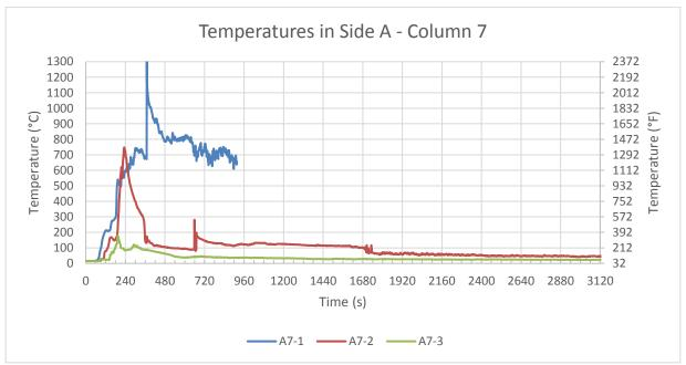
Figure B-42: Test 2 temperatures in Side A: Column 7. Note that TC A7-1 malfunctioned during the test and suspect data have not been plotted, additionally, it exceeded the maximum rating of a Type K TC at 06:10 after which time the temperature decreased. Its functionality was checked post-test and found to be inoperative. Note different temperature scale.
