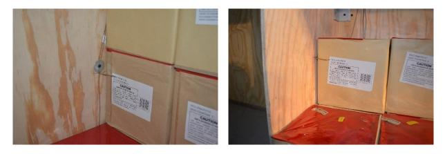
Figure 2-27: TC installation in shelving units (a) TC along perpendicular flame break, (b) TC located on transverse flame break. TCs located such that bead is 5.1 cm (2 in.) from the flame break.
