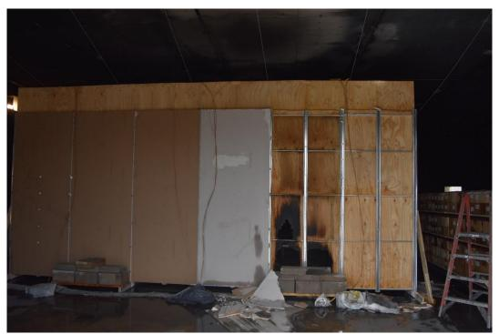
Figure C-8: Test 1 damage to Side C. Showing back of Side C where sheet rock has been removed post-test to inspect the burn through of the longitudinal flame break.
