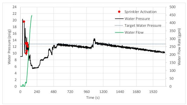
Figure 3-2: Test 1 water pressure and flow rate.
