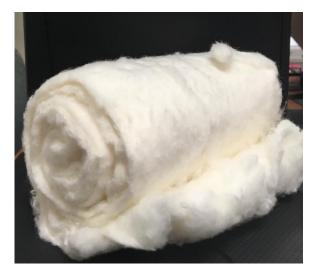
Figure 2-23: Standard full cellucotton ignitor (without bag and gasoline).
