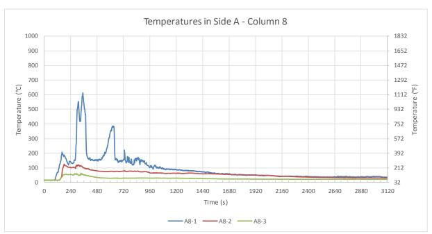
Figure B-43: Test 2 temperatures in Side A: Column 8.
