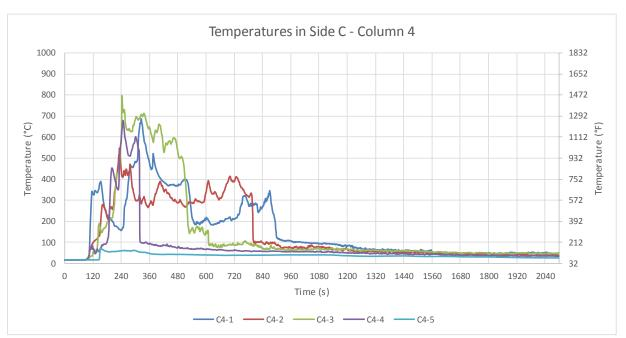
Figure B-23: Test 1 temperatures in Side C: Column 4.
