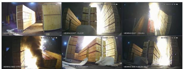
Figure A-23: Test 2 at 01:20: fire and smoke production intensifying in Side A, sparks being projected throughout lab space and showering down on top of Side B, Side C ignited at 01:19.
