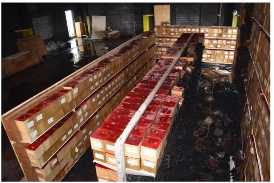
Figure C-3: Test 1 overview of damage looking toward east. Commodity shown collapsed into the aisle between Sides A and C.
