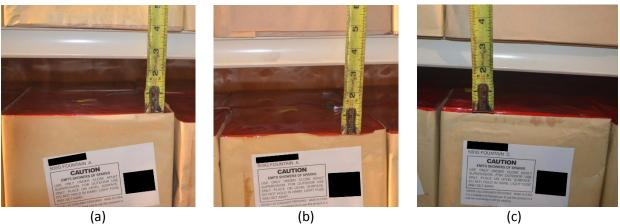
Figure 2-20: Air gap between top of commodity and underside of shelf above for (a) bottom shelf commodity in Side A, B, D, and E, (b) middle shelf commodity in Side A, B, D, and E, and (c) commodity in all shelves of Side C.
