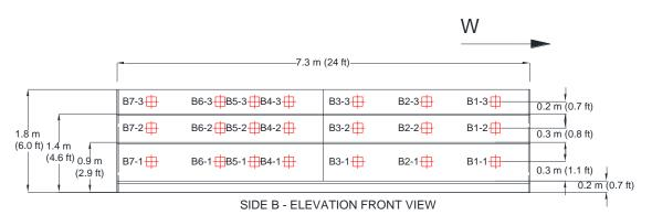
Figure 2-4: Front elevation view of Side B showing shelf height and thermocouple nomenclature and vertical dimensions of locations. Red crosses represent TCs.
