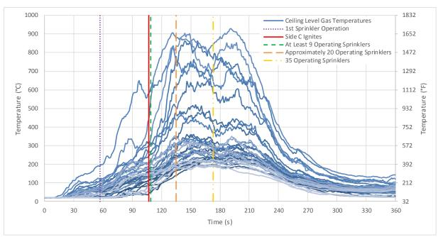
Figure 4-1: Test 1 ceiling-level gas temperatures and relevant events.
