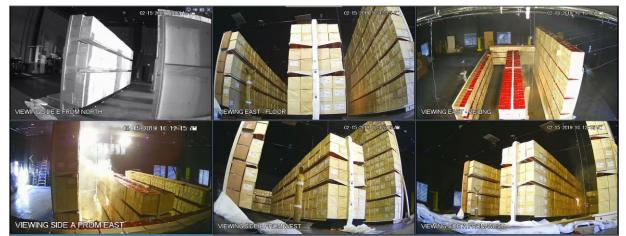
Figure A-1: Test 1 at 00:40: flames present on the face of Side A at ignition location.
