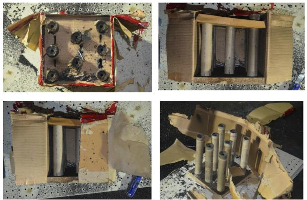
Figure 2-15: Discharged fireworks device that has been deconstructed showing engineered wood product base and cellulose tube and outer construction with red colored cellophane sheet on top.
