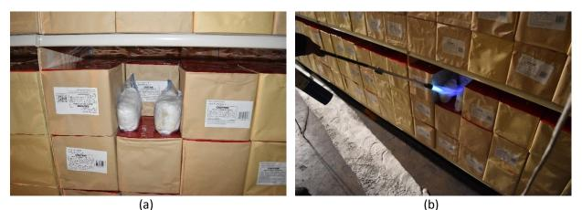
Figure 2-24: Ignition within the test array (a) close up showing ignitor placement, (b) ignition by application of propane torch.
