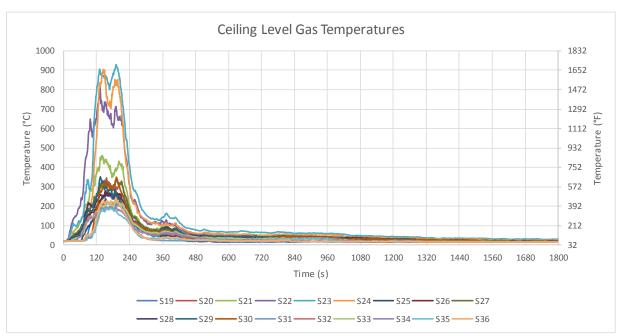
Figure B-2: Test 1 ceiling-level gas temperatures at TC locations 19-36.
