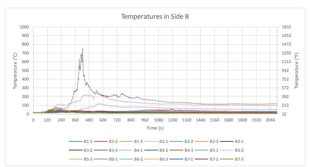
Figure B-15: Test 1 temperatures in Side B. Elevated temperatures are witnessed in the absence of fire on Side B. The longitudinal flame break on Side B had been minorly breached allowing the transport of hot gases. Refer to Section C.1 in Appendix C.
