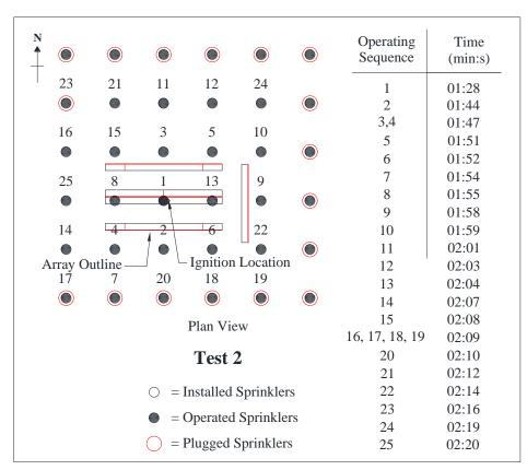
Figure 3-6: Test 2 sprinkler operation pattern. Note that northern and eastern most rows of sprinklers were not electronically monitored for their operation time.
