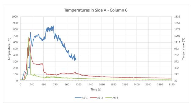
Figure B-41: Test 2 temperatures in Side A: Column 6. Note that TC A6-1 malfunctioned during the test and suspect data have not been plotted. Its functionality was checked post-test and found to be inoperative.
