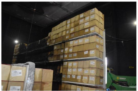
Figure C-25: Test 2 Side C, east side on left, west on right, shelves 3-5, fire damage reached transverse flame break on west side of shelf 3 but did not burn through and flame front ceased on west side of shelves 4 and 5 prior to reaching transverse flame breaks.
