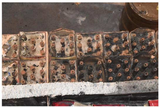
Figure C-28: Test 2 Side B detail of fire damage, a total of 22 fireworks devices became active in this location.
