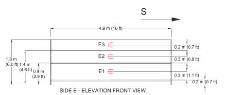
Figure 2-7: Front elevation view of Side E showing shelf height and thermocouple nomenclature and vertical dimensions of locations. Red crosses represent TCs.
