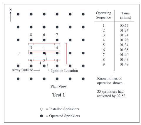
Figure 3-1: Test 1 sprinkler operation pattern. Note that only 9 of 36 sprinklers were electronically monitored for their operation time.
