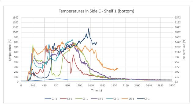
Figure B-45: Test 2 temperatures in Side C: Shelf 1 (bottom). Note that TCs C3-1, C4-1, C5-1, C6-1 and C7-1 malfunctioned during the test and suspect data have not been plotted. Their functionality was checked post-test and found to be inoperative. Note different temperature scale.
