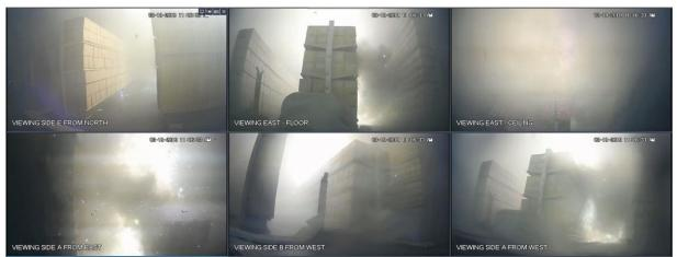
Figure A-28: Test 2 at 02:10: at least 20 sprinklers operating, fire continues to intensify and visibility is becoming more obscured.
