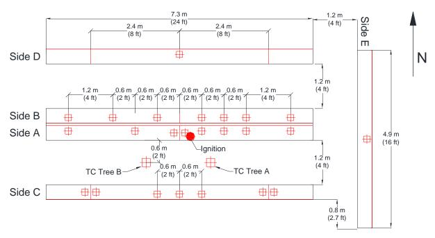
Figure 2-1: Plan view of shelving unit layout indicating nomenclature of sides and with thermocouple locations (red crosses).
