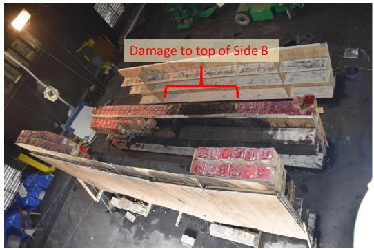
Figure C-27: Test 2 shown from aerial perspective with commodity partially removed and highlighting location on Side B where fire damage was sustained.
