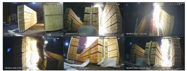
Figure A-22: Test 2 at 01:10: fire and smoke production intensifying in Side A.
