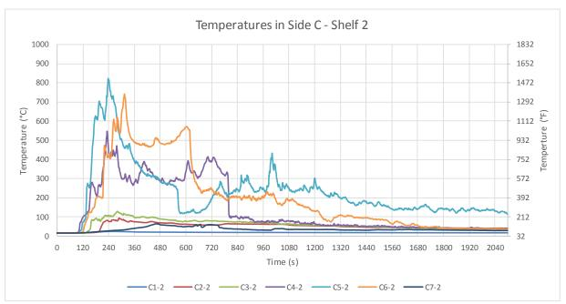
Figure B-17: Test 1 temperatures in Side C: Shelf 2.
