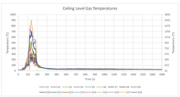
Figure B-30: Test 2 ceiling-level gas temperatures at TC locations 1-18.
