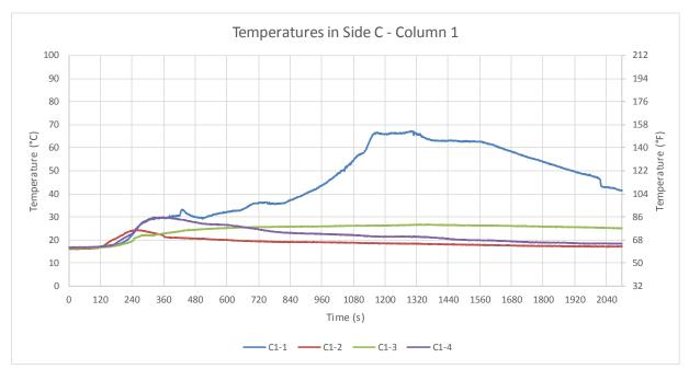
Figure B-20: Test 1 temperatures in Side C: Column 1. Note different temperature scale.
