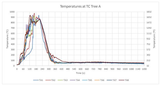
Figure B-28: Test 1 temperatures at TC Tree A. High temperatures are a result of the proximity of the fire to the TC tree and are not indicative of vertical temperature profiles in other regions of the test array.
