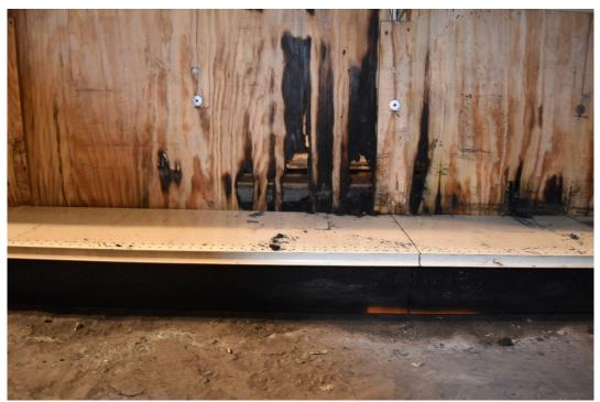
Figure C-30: Test 2 Side B after commodity has been removed showing localized area of burn through of longitudinal flame break in bottom shelf behind ignition region.
