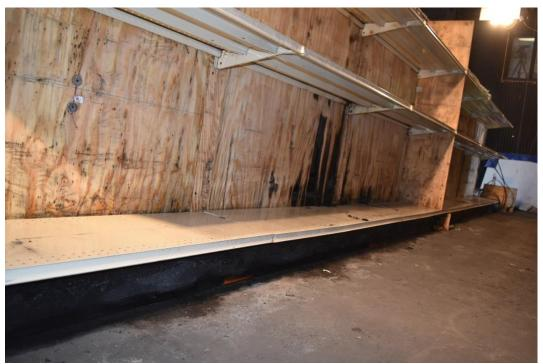
Figure C-29: Test 2 Side B after commodity has been removed showing localized area of burn through of longitudinal flame break in bottom shelf behind ignition region. See Figure C-30 for a close up image of this burn through.
