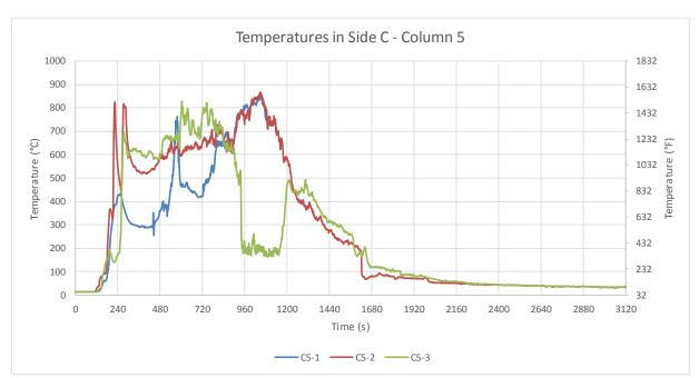
Figure B-53: Test 2 temperatures in Side C: Column 5. Note that TC C5-1 malfunctioned during the test and suspect data have not been plotted. Its functionality was checked post-test and found to be inoperative.
