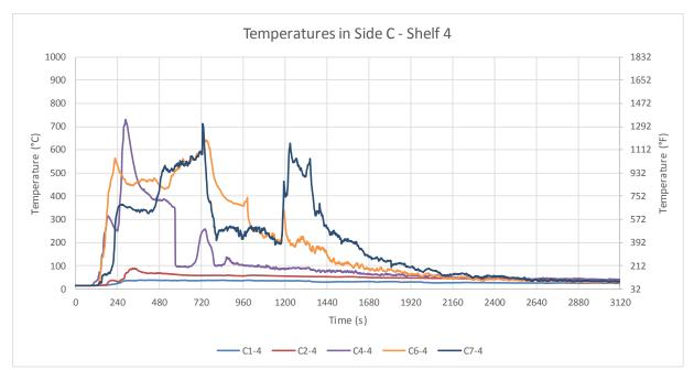
Figure B-48: Test 2 temperatures in Side C: Shelf 4. Note that TC C4-4 malfunctioned during the test and suspect data have not been plotted. Its functionality was checked post-test and found to be inoperative.
