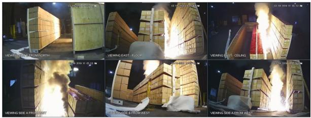
Figure A-21: Test 2 at 00:50: fire and smoke production intensifying in Side A with flames extending approximately 2.1 m (7 ft) above top of commodity.
