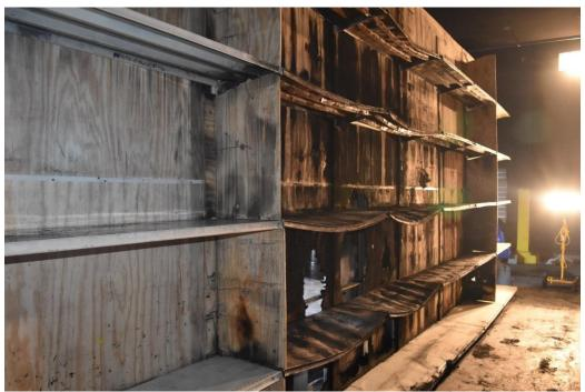
Figure C-17: Test 1 Side C (looking westward) after commodity has been removed showing transverse flame breaks intact, localized burn through of longitudinal flame break, and deformation of metal shelves.
