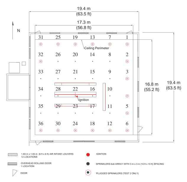
Figure 2-26: Plan view of test array and ceiling-level sprinklers within the laboratory space. Numbering above each sprinkler location is also associated with the TC at each location.
