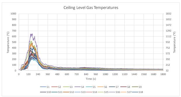
Figure B-1: Test 1 ceiling-level gas temperatures at TC locations 1-18.
