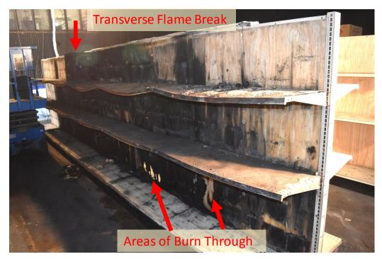
Figure C-32: Test 2 Side A (looking westward) after commodity has been removed showing transverse flame breaks on bottom and middle shelves consumed but intact on top shelf, examples of burn through of longitudinal flame break, and deformation of metal shelves.
