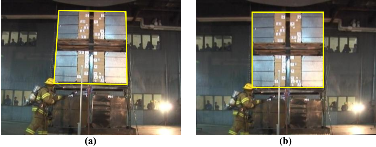
Figure 4-21: Example of perspective correction. (a) Uncorrected image and (b) image after correction
