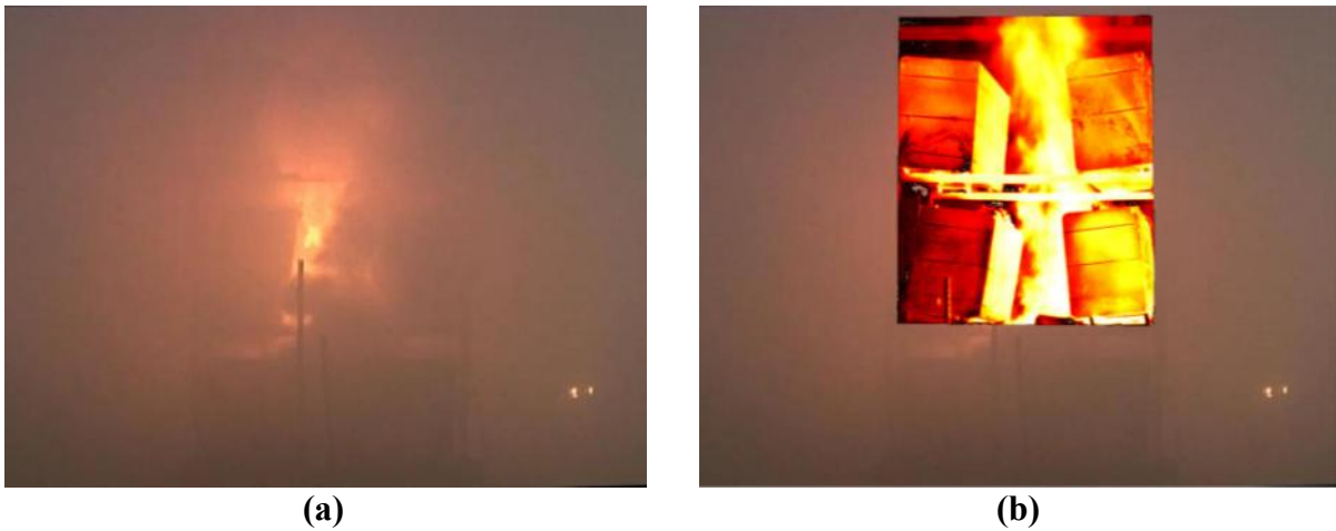
Figure 4-23: Example of the LWIR camera's ability to see through smoke and steam. (a) Visual image and (b) IR image registered on the top two tiers
