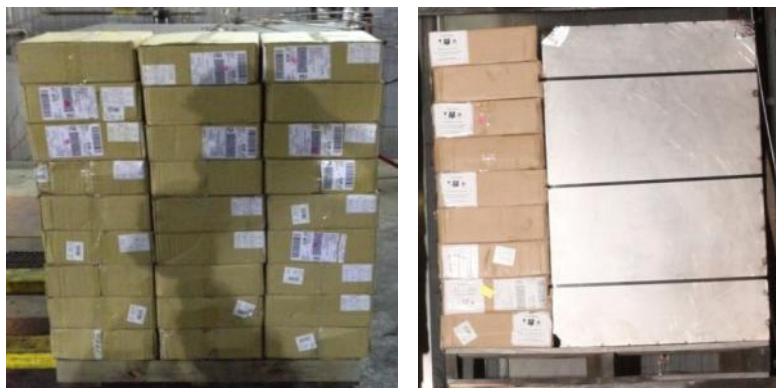
Figure 4-15: Pallet design for Li-ion polymer cells
