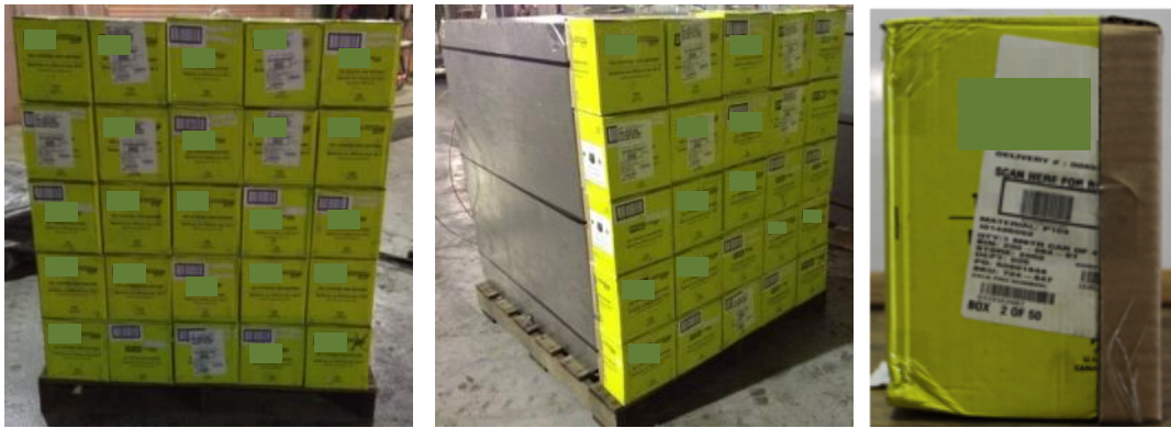
Figure 4-11: Pallet design for Li-ion power tool packs
