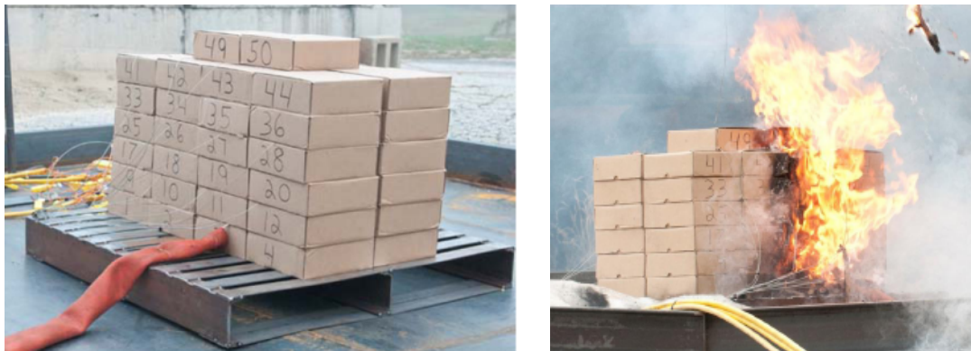
Figure 6-1: Image of 5,000 Li-ion battery test conducted by the FAA; test layout (left) and fire involving carton packaging (right) [images taken from reference 8]
