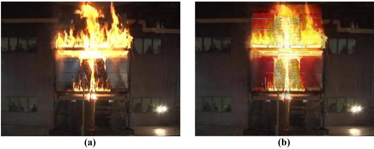
Figure 4-22: Example of IR image registration. (a) Visual image and (b) IR image registered on the top two tiers
